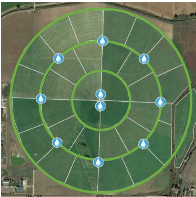
Figure 6. MiG system design on a 200-acre pivot including high-tensile concentric fences (green), moveable polywire paddock fencing (white), and watering locations at Colorado State University. Polywire locations represent areas associated with given water points and are often further subdivided into 2 or 3 smaller paddocks depending on animal numbers and current forage supply (Figure by Casey Shawver, retrieved from PastureMap mobile application).
